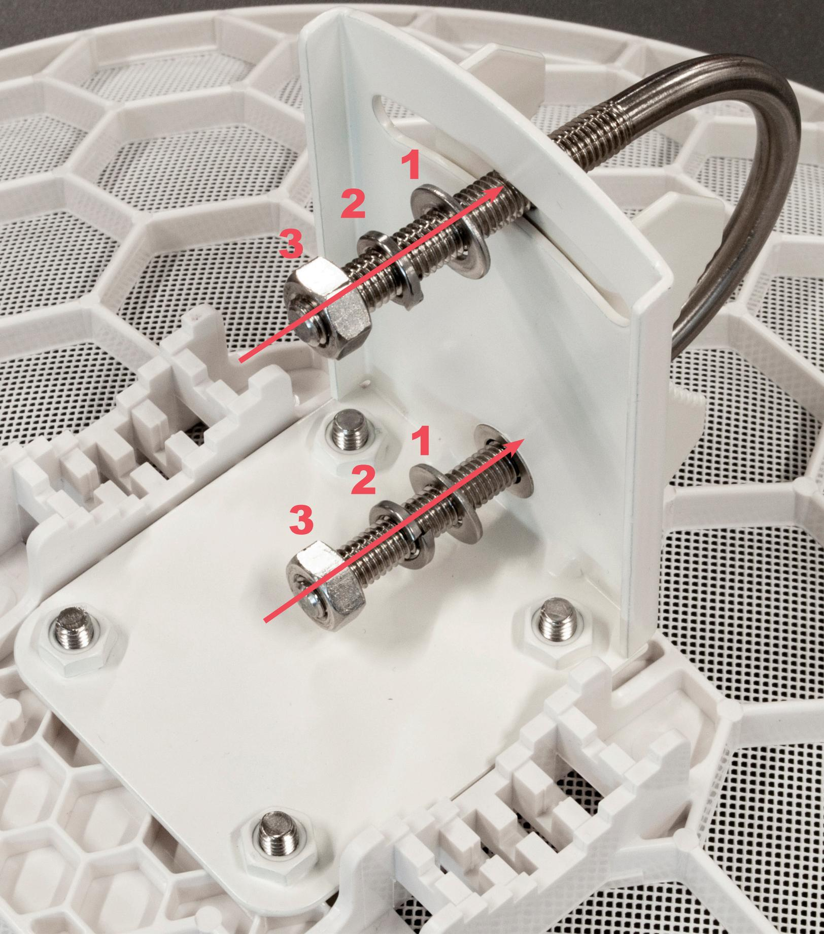
**5** Use the provided M8 washers and nuts in the order that is specified in the image. Tighten the nuts with the 1/2 wrench.
