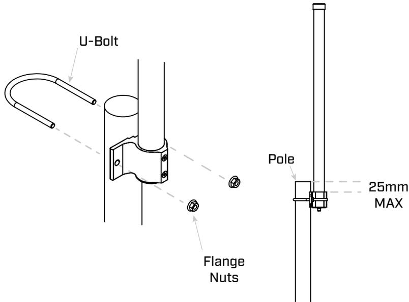
Place the antenna against the tip of the pole. Attach the U-Bolt to the pole and place it through the mounting holes of the antenna. Use the included Flange Nuts to secure the antenna in position. Compatible with pole sizes from 25-50mm. Best performance will be achieved if antenna is mounted less than 25mm from the top of the pole.
