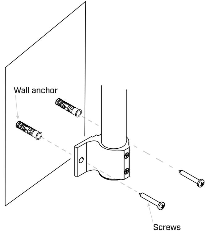
Place the antenna against the wall, mark the mounting holes. Put down the antenna and drill two 4mm holes, press the wall anchors in them. Place the antenna and fix the screws. Best performance will be achieved if antenna is mounted less than 25mm from the top of the wall.
