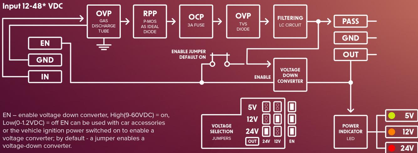
EN – enable voltage down converter, High(9-60VDC) = on, Low(0-1.2VDC) = off EN can be used with car accessories or the vehicle ignition power switched on to enable a voltage converter; by default - a jumper enables a voltage-down converter.
