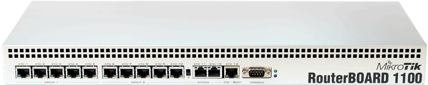
The RB1100 is a rackmount router with 13 Gigabit Ethernet ports. Two of the ports provide bypass functionality. There are two models, a dual core 1066MHz PPC processor and 1GB of RAM (RB1100Hx2), or with a dual core 1066MHz PPC processor with hardware encryption and 2GB of RAM (RB1100AHx2).
