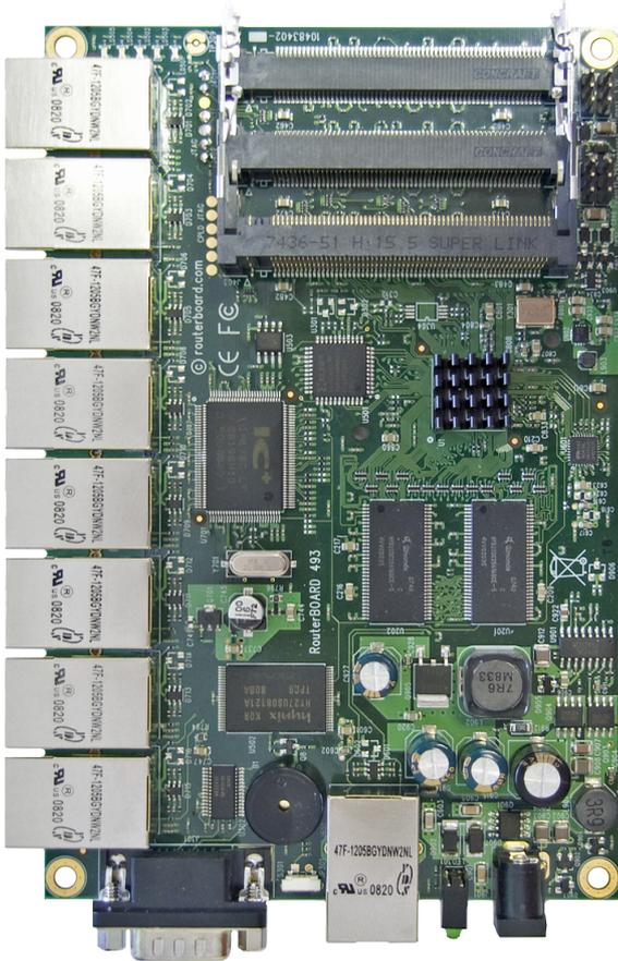
The RB493 has nine ethernet ports and three miniPCI slots, it also has a switch chip, so the ethernet ports of your choice can be grouped together to make it act as a switch.
