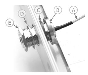
The N-female antenna "pigtail" connector is assembled on the case, as shown on the picture to the left. The red rubber ring  ${\bf C}$  is put on the connector  ${\bf B}$ , then the connector is inserted into the appropriate hole of the waterproof case (from inside the case), and secured reliably with the nut  ${\bf E}$  and lock washer  ${\bf D}$  from outside of the case.
